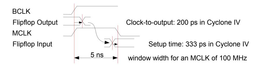
Using the rising edge of MCLK is unreliable because of clock jitter!
